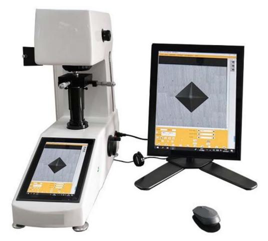
PCHVT-50Z is a new generation of Vickers hardness tester adopts the integrated design of hardness tester and panel computer, all the testing parameters can be selected on the panel computer.
